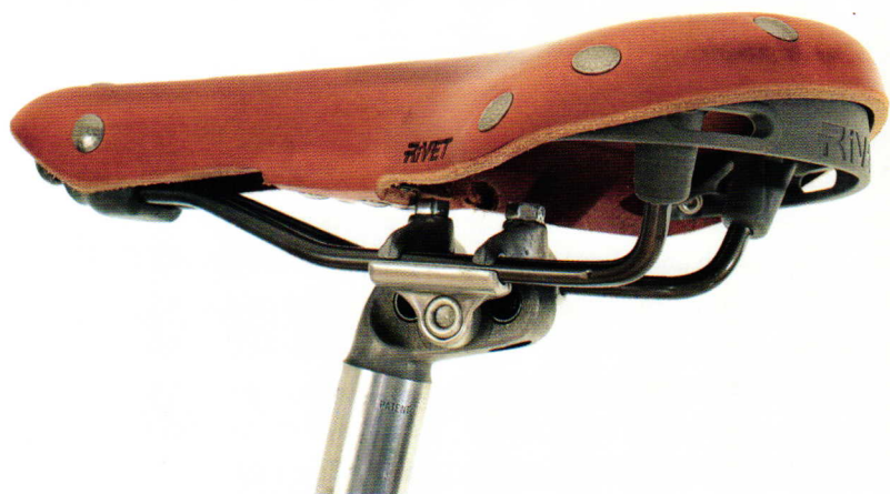
Bottom: Toward the end of this test, the saddle had stretched significantly. Re-tensioning the saddle for the second time straightened the top again.
